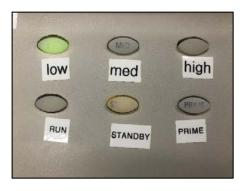
Run: Pressurizes the tube, allowing for sample to be acquired.
